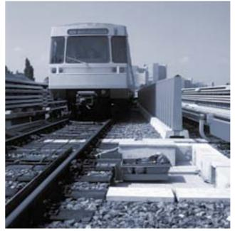
Picture 4: Points Machine along the tracks.
